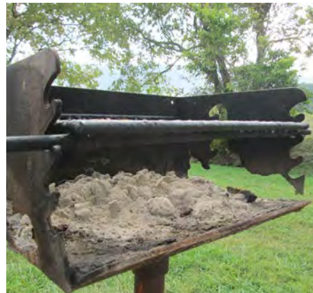
Grill rusting out
