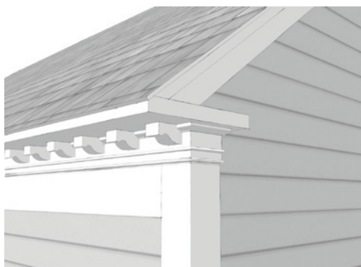
A classical cornice with modillion blocks.
