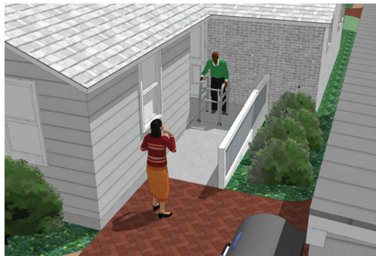
Side entrances with driveway access can be sensible choices for creating handicap accessible entries.
