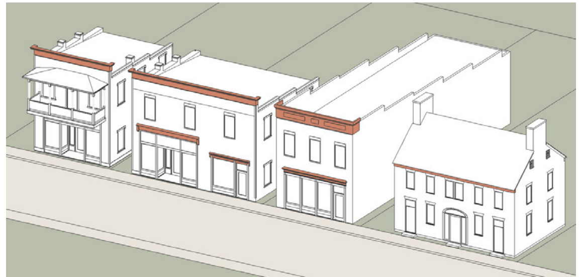
Cornice are a defining feature of commercial structures in the district.
