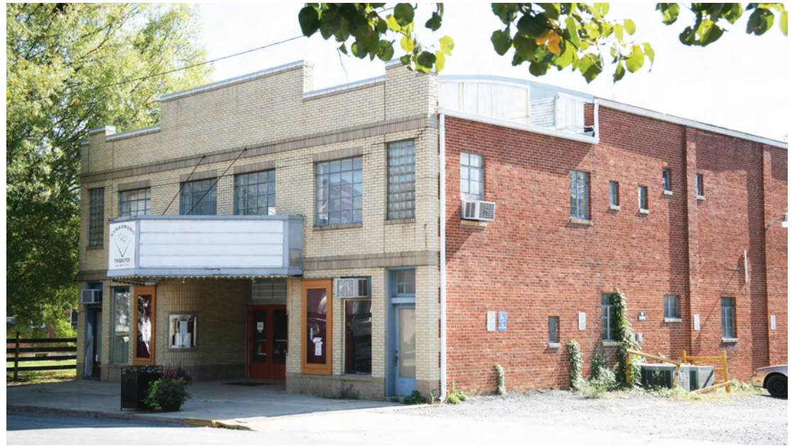
The Theatre at 151 West King Street displays elements of this style including a simple two-toned brick facade with small-paned, metal-framed windows and glass-block-filled openings. A stepped parapet above the roofline and contrasting darker color brick banding emphasize the horizontal nature of the facade.
