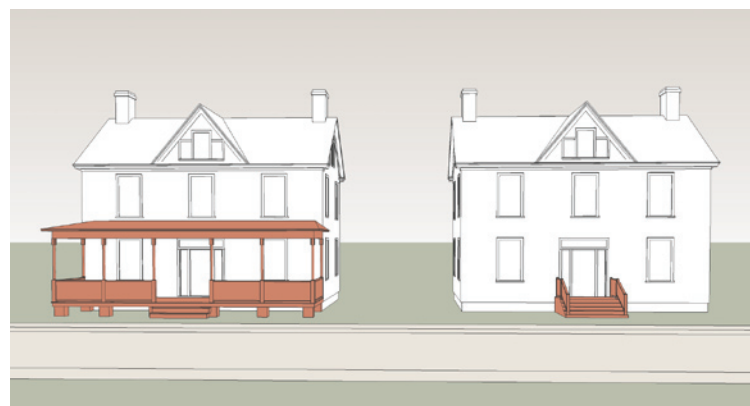
A side-by-side comparison of the same house with and without a porch shows how a porch can be used to reduce the perceived size of the structure and relate it to a human scale.
