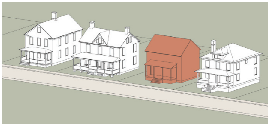
An APPROPRIATE example of mass for new construction relates to adjacent house forms
